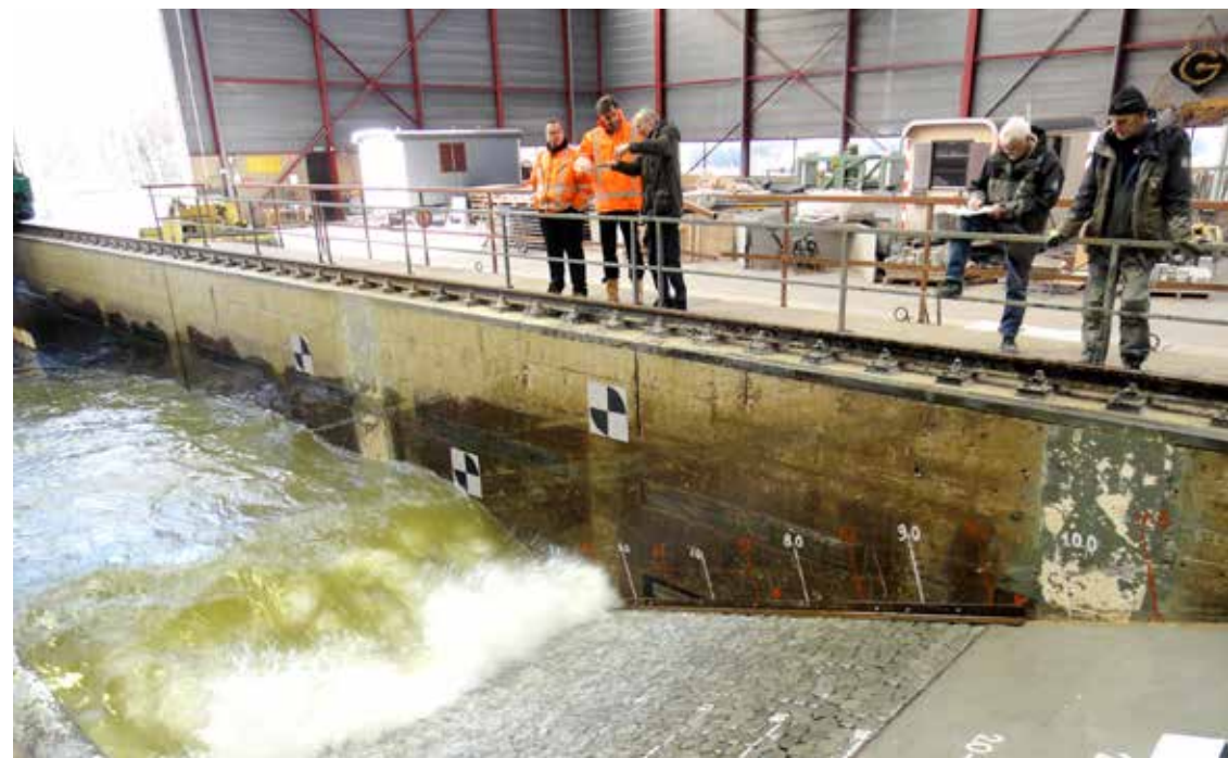
Zetstenen testen in de Deltagoot in Delft
